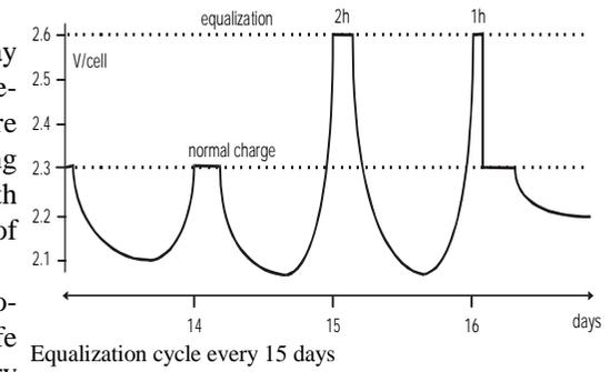
To prevent this separation of electrolytes and to improve the battery life span, the SLR130/145 starts every fifteen days a gassing cycle. For about three hours the final charge voltage will be increased to 2.6V/cell. The resulting gassing phase will be finished after three hours of gassing charge (>2.4V/cell). (See figure)
